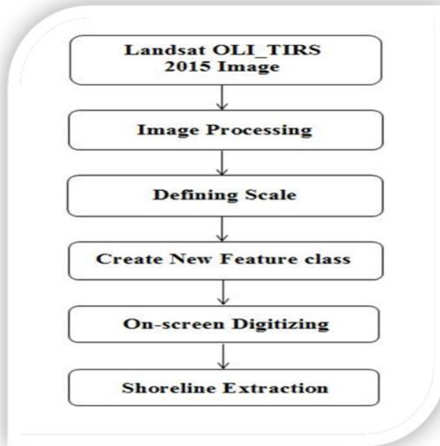
Fig. 3. Methodology to extract shoreline using on-screen digitizing method
